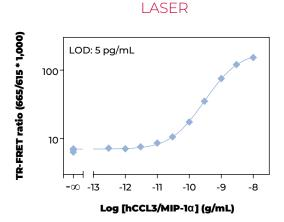
Figure 3 Typical nonlinear human CCL3/MIP-1α standard curves in Assay Buffer 1. Left: lamp excitation, Right: laser excitation. Data represent the mean ± standard deviation of triplicate measurements (3 wells) for each standard. The data was generated using a low-volume 384-well white plate read on the EnVision® equipped with TR-FRET option.
