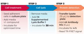
Figure 2 Assay workflow using the 2-plate (transfer) protocol.
