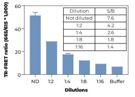
Quality Control: the Phospho-4EBP1 (T37/T46) + Total 4EBP1 assay kit is routinely tested against A431 lysates. A431 cells were cultured in a T175 flask to 70% confluence. Following cell lysis using 4 mL of 1X Lysis Buffer 2, lysates were serially diluted with 1X Lysis Buffer 2 and tested in triplicate and in separate wells for phospho-4EBP1 (T37/T46) and total 4EBP1. Data show a linear relationship between lysate dilutions and TR-FRET ratio values.
